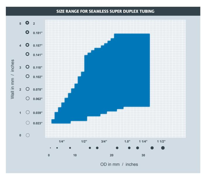
Our tubing sizes typical for Super Duplex range from: **3.18 mm (0.125 in) to 31.75 mm (1.25 in)** outer diameter OD in seamless form.
